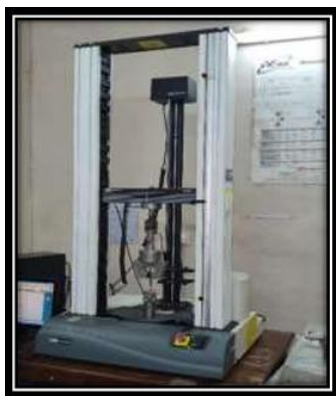
FIG 13: Specimen subjecting to compressive loading
