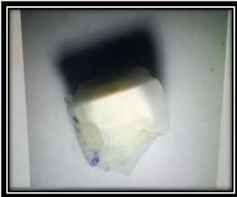
FIG 12: Extent of dye penetration
